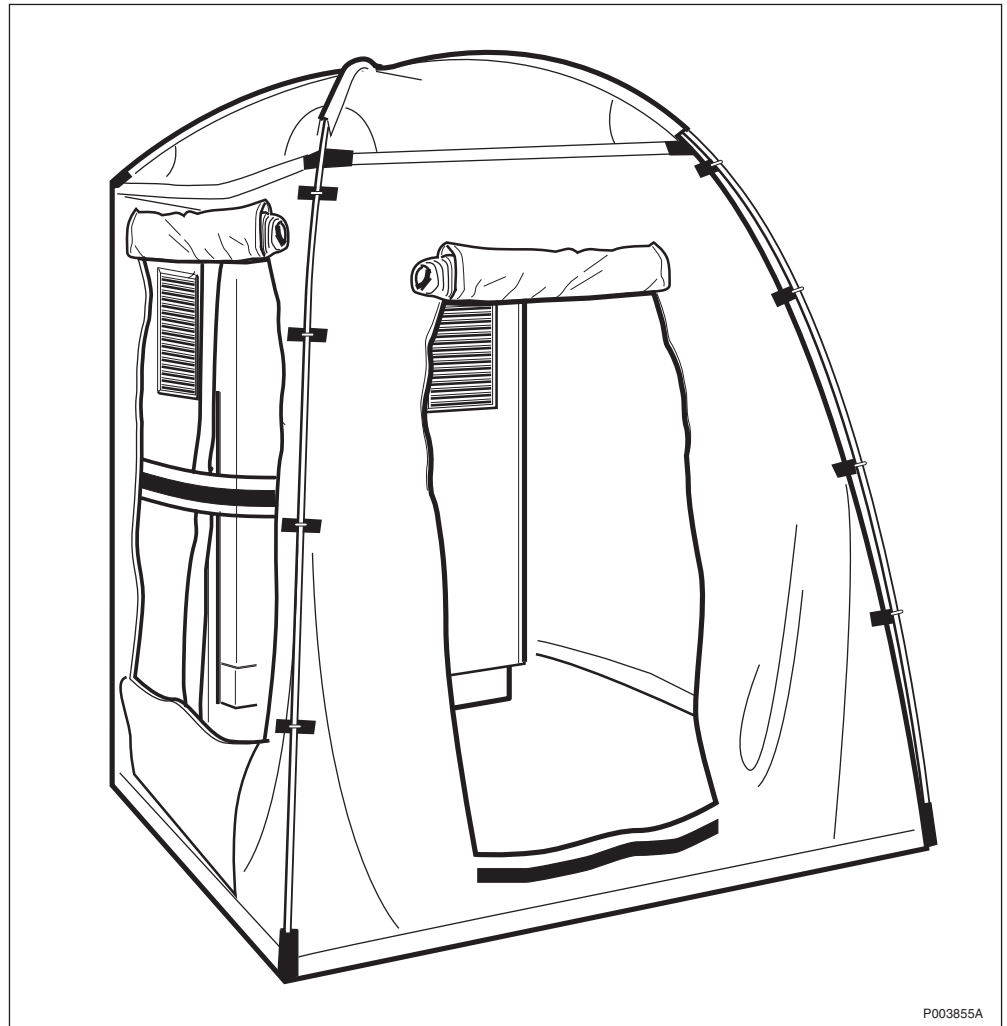
Figure 21 Shutters for the Climate Unit vents
