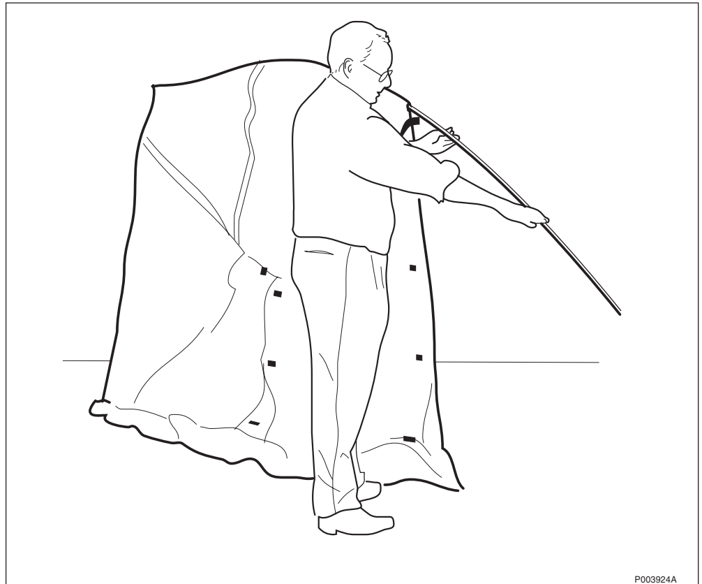
Figure 14 Roof tent-pole insertions
